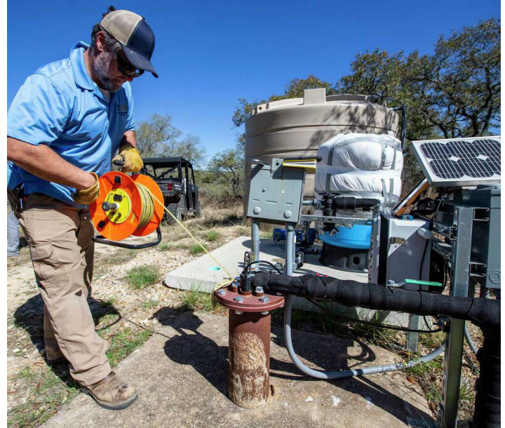
Charles Crawford, data collection supervisor at the Edwards Aquifer Authority, measures the water height of a well at the authority's Field Research Park in far north San Antonio. Photo: William Luther
