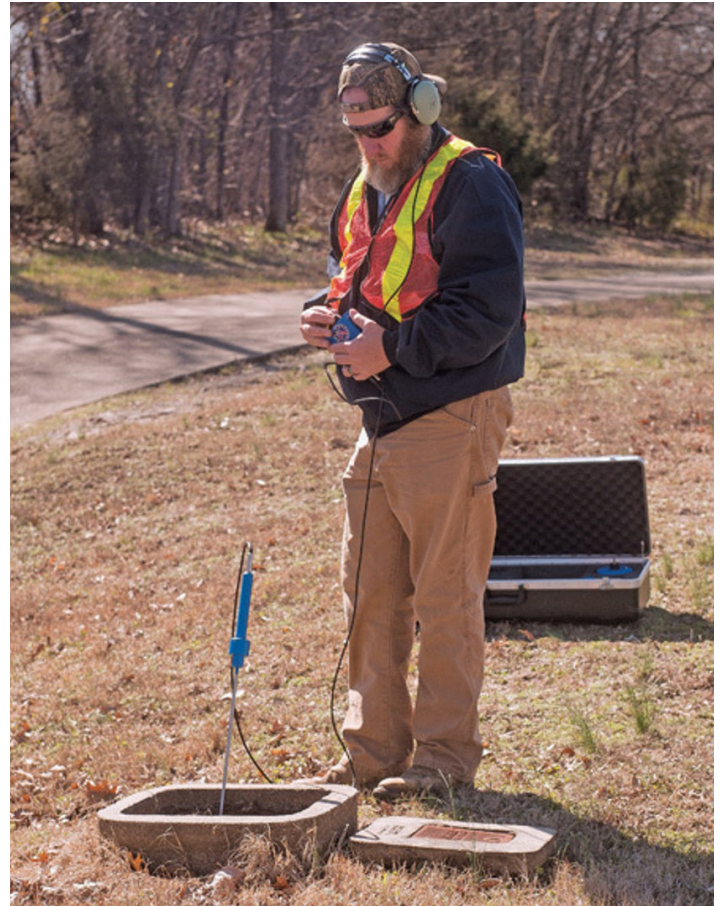
Figure B-7. B.J. Baugus uses an Aqua-Scope leak detector to help pinpoint a leak in the Wilson County water system. Photo: Peter Kenter, Municipal Sewer & Water
