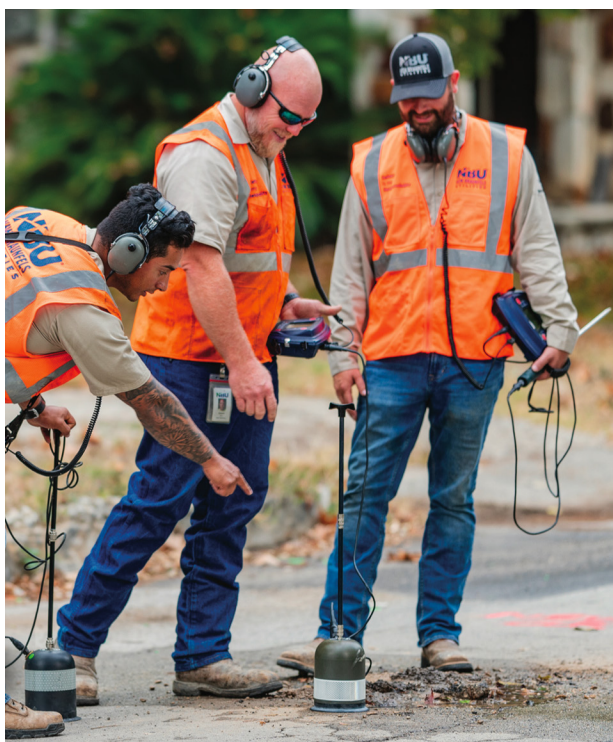
Left: A leak detection crew at work with acoustic leak detection equipment in New Braunfels, Texas. Photo: Peter Kenter. Below, clockwise starting from top left: a small customer meter, large customer water meter, electronic controller, and a pressure reducing valve.
