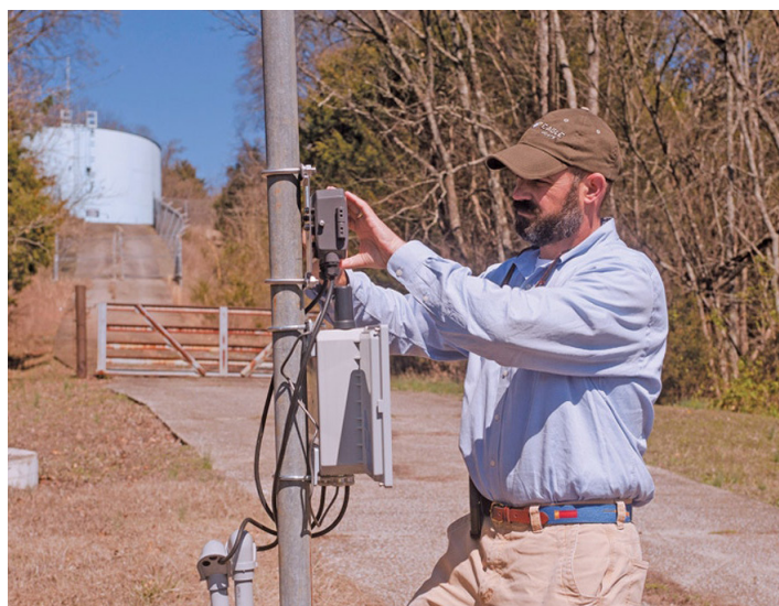
Chris Baenziger checks the ultrasonic flow meter at a storage tank in Wilson County, Tennessee. Photo: Peter Kenter
